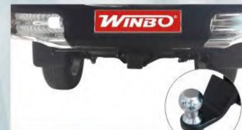
PW015558 BLACK REAR HITCH FOR VEHICLE W/ OE REAR BUMPER WITHSTANDS TENSION OF 6000 LBS
