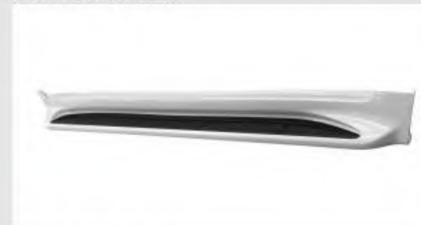
PW018124 ELEGANCE STYLE RUNNING BOARD PW00456230 NEED TO INSTALL WITH MUD FLAP
