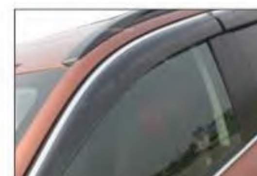
PW00396112 RAIN SHIELD
