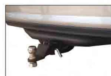
PW018736 REAR HITCH WITH RECEIVER & BALL WITHSTAND THE TEMSION OF 6000LBS
